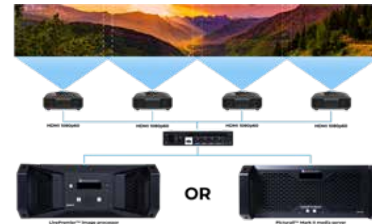
Example 3: one 8Kx1K@60Hz input to four 1080p projectors
